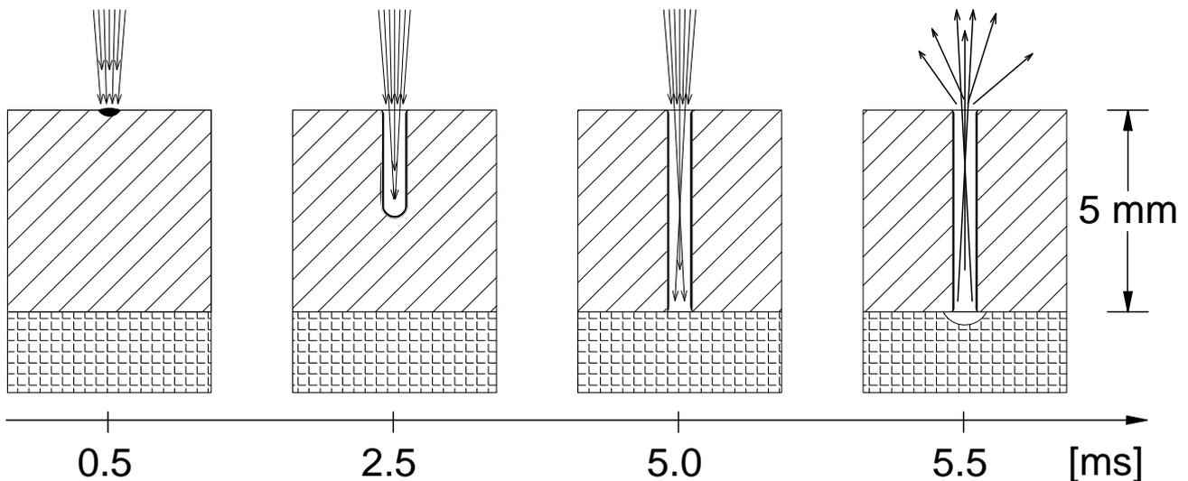
The principle of EB drilling
