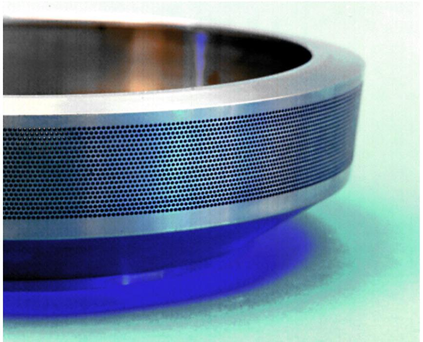
Spinner used in glass fibre production 47.45.01b/7
