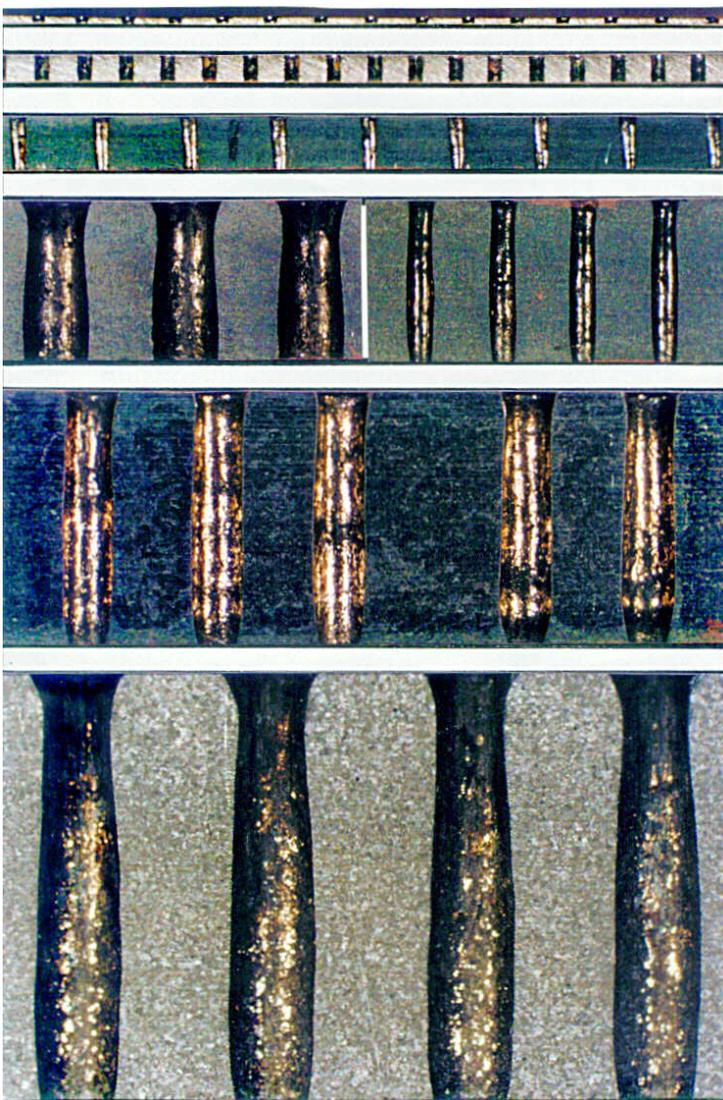
Cross-sections of EB drill-holes
